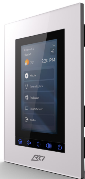
The KX4 hard buttons (5) may be custom laser etched using the RTI Laser Shark service.
