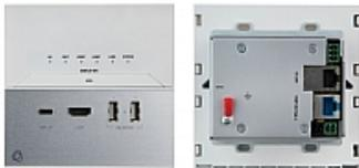
EXT3-C-WP-XR-T USB-C transmitter is a high-performance, extended-reach HDBaseT 3.0 transmitter for 4K60Hz (4:4:4) HDMI, USB, Ethernet, RS-232, and IR signals over twisted pair. The EXT3-C-WP-XR-T transmitter converts all input signals into the transmitted HDBaseT 3.0 signal and extends it over HDBT to a compatible receiver. The EXT3-C-WP-XR-T transmitter accepts power over the copper extension cable from a PoE provider remote device
