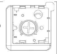
If the screen locks at the bottom and will not retract, turn adjustment knob one quarter turn counterclockwise.
